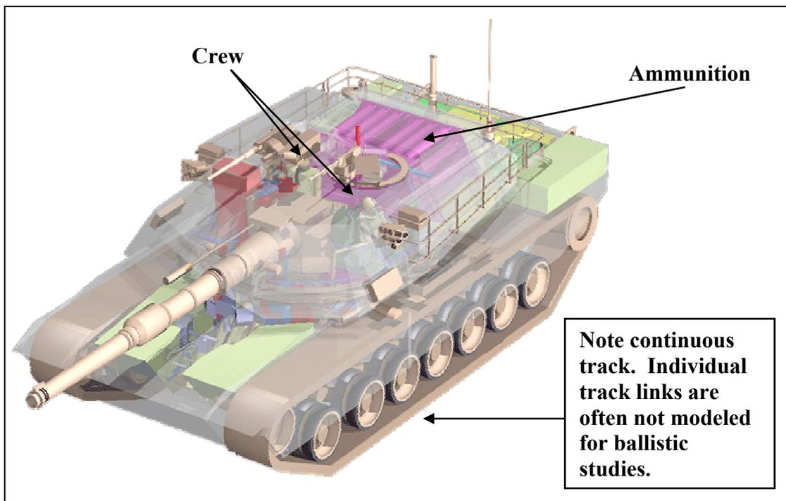
Figure 1. Ballistic penetration model with transparent exterior.
