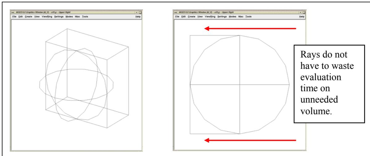
Figure 14. Example of a compact bounding primitive.
