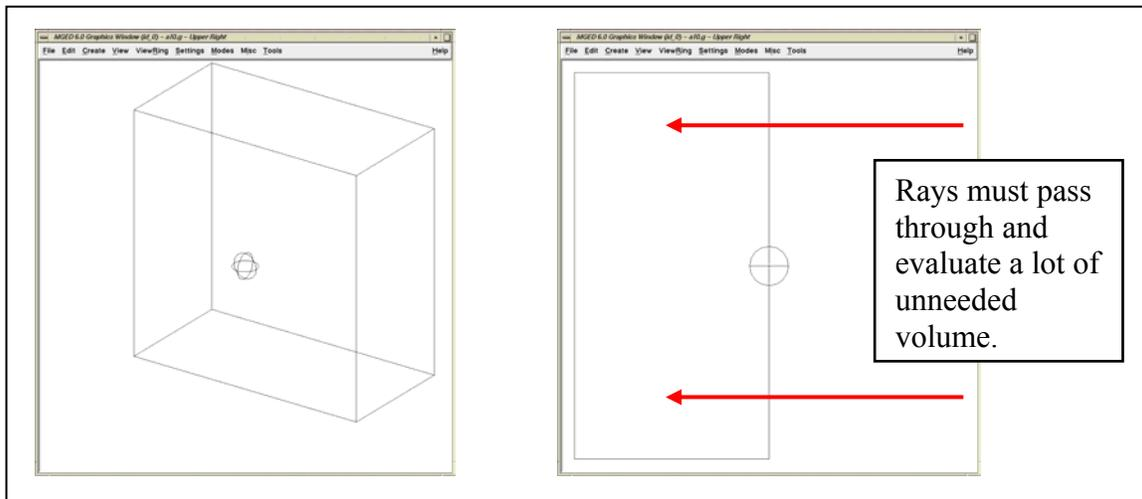
Figure 13. Example of an Overly Large Bounding Primitive.
