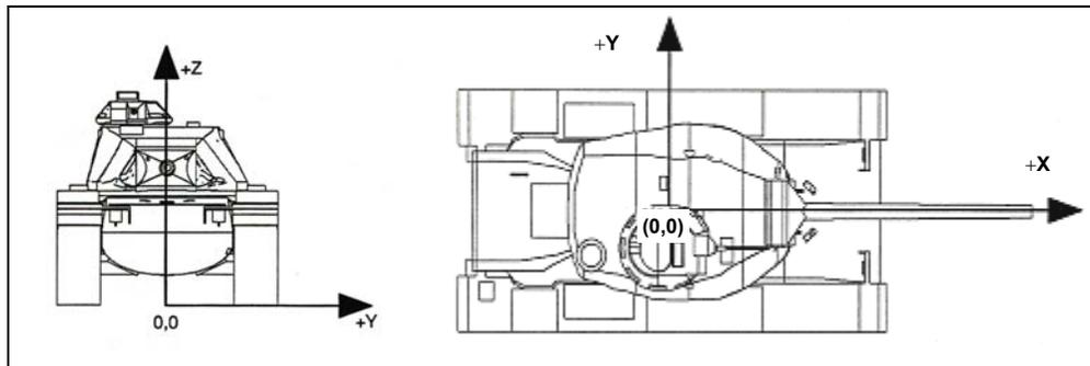
Figure 6. Coordinate axes of a turreted ground vehicle.
