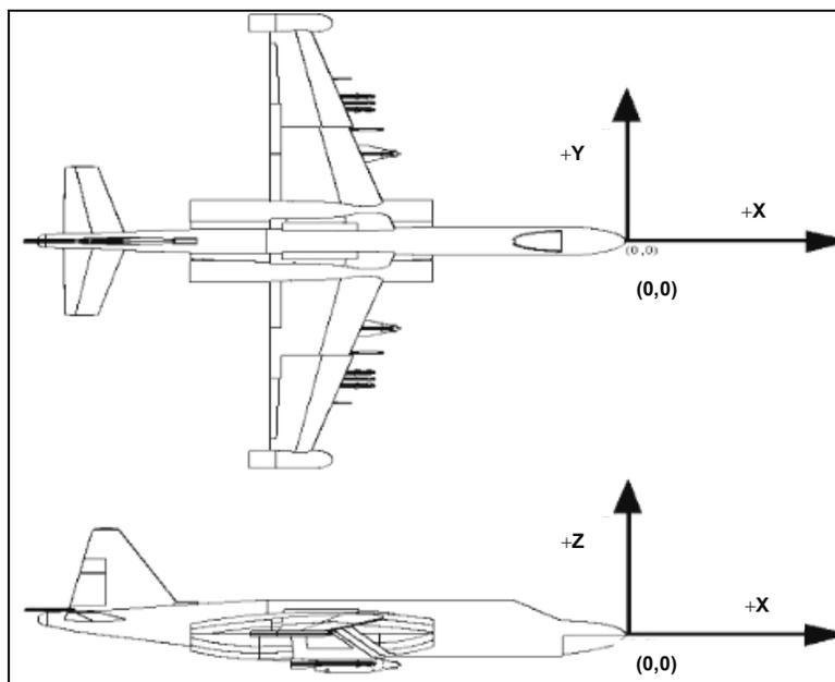
Figure 8. Coordinate axes of a fixed-wing aircraft.
