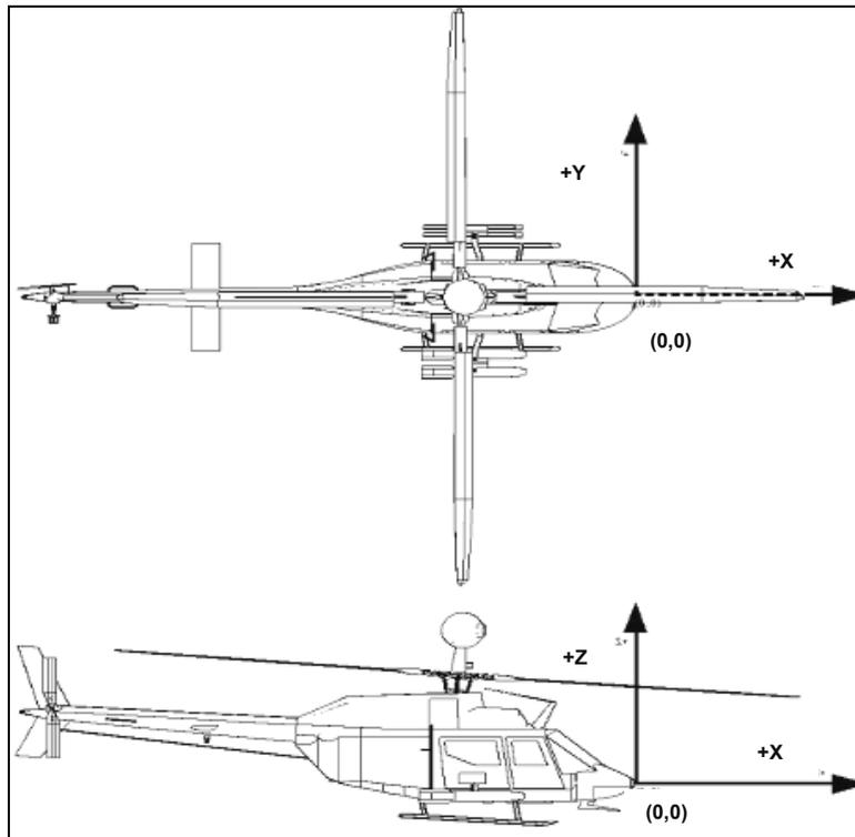
Figure 9. Coordinate axes of a rotary-wing aircraft.
