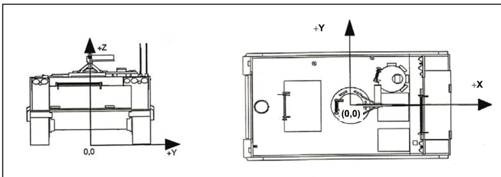
Figure 7. Coordinate axes of a nonturreted ground vehicle.
