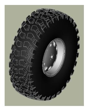
External view of a 395/85R20 tire with off-road tread and deepened tread grip.
