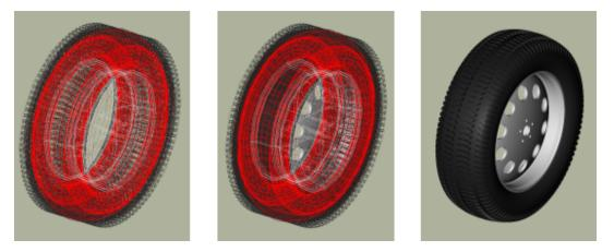
Combination of curved profile, off-road tread and increased tread pattern count - generated by tire -p 2 -t 1 -c 100
