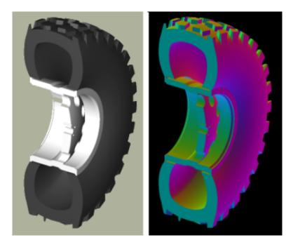
Cross section views - default and surface normal - of the new 395/85R20 tire with increased thickness.
