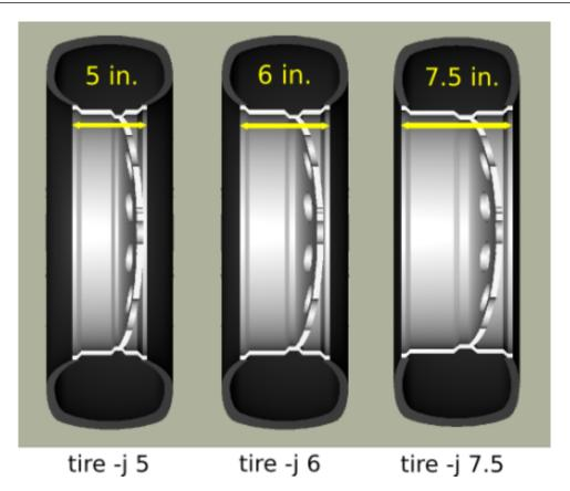
Demonstration of tire model changes when different rim widths are used.
