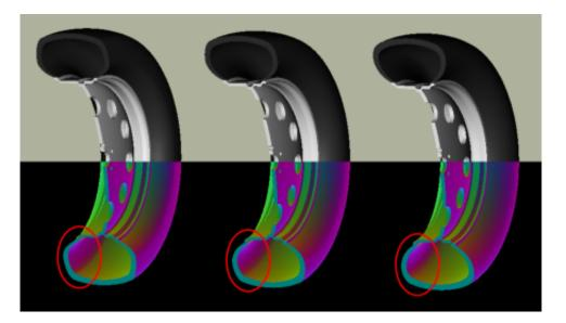
From left to right, the *s* flag settings are 260, 270 and 280. Notice in the surface normal view the change in color gradient on the side walls, and in the normal view notice the different shapes the tires exhibit. The visual impact of this parameter can be fairly subtle.
